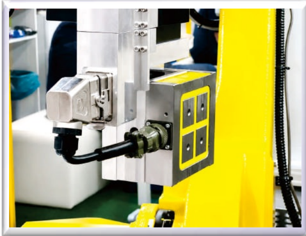
方形永磁式電控夾頭 Electro-Permanent Magnetic Chuck for Automatic Robotic Arm
